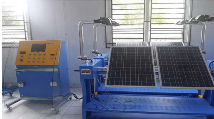
Figure 6. Solar Module Characterization Instrument
