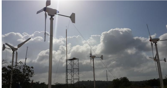
Figure 8. Total 8 kW wind energy converter HAWT
