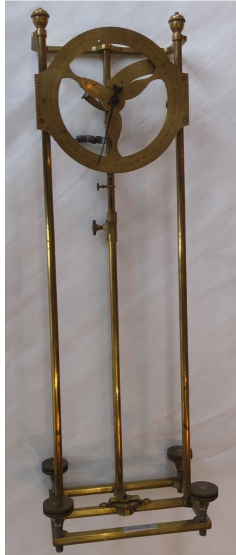
Fig. 1: Hair hygrometer, front side, in lying position (which is not the intended one for using the instrument). Source: Deutsches Museum (inventory number 128). Photograph taken by the author.
