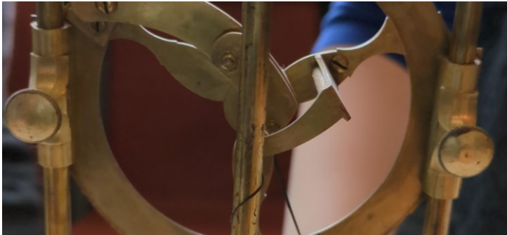
Fig. 2: Hair hygrometer, close-up of the back side of the scale and the two hand screws to adjust its height. Source: Deutsches Museum (inventory number 128). Photograph taken by the author.
