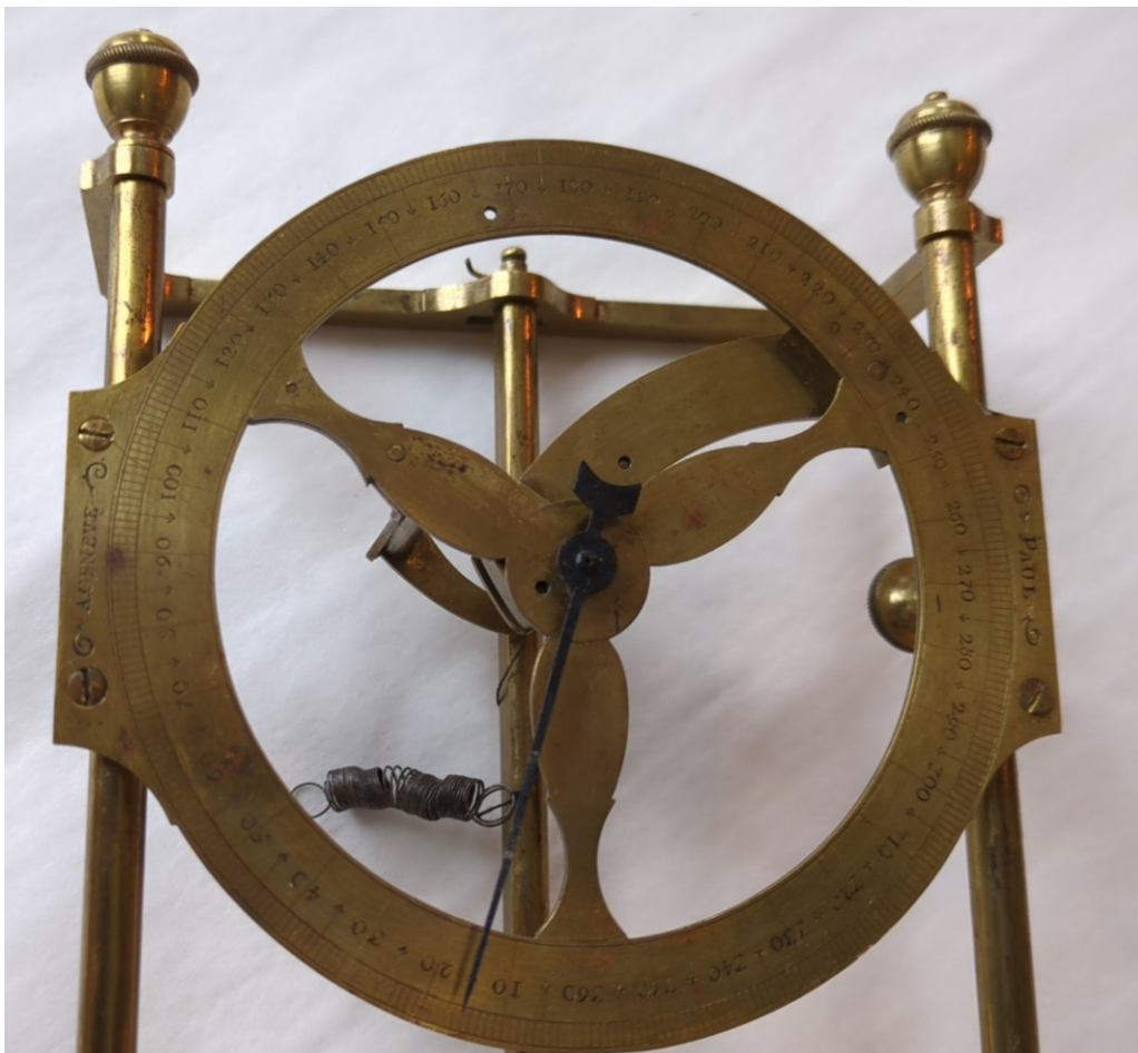
Fig. 3: Hair hygrometer, close-up of the circular scale, from the front. In the background the (non-original) metal spring. Source: Deutsches Museum (inventory number 128). Photograph taken by the author.
