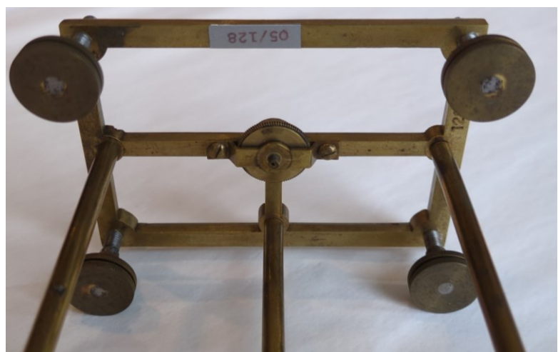
Fig. 10: Hair hygrometer, close-up of the bottom frame with the flat gear in its centre. Source: Deutsches Museum (inventory number 128). Photograph taken by the author.
