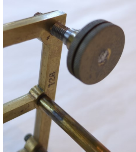
Fig. 11: Hair hygrometer, close-up of the black inventory number on the bottom frame. In the foreground one of the four probably non-original hand screws. Source: Deutsches Museum (inventory number 128). Photograph taken by the author.
