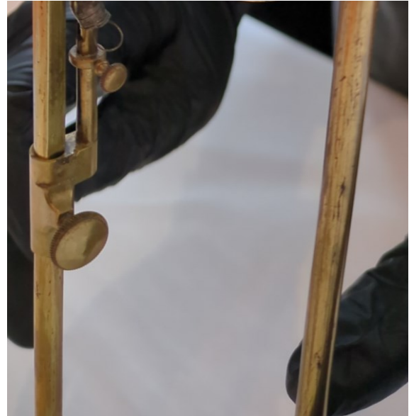
Fig. 8: Hair hygrometer, from the back, close-up of two vertical bars. One with hook and flattened part. Signs of damage and oxidation on the other bar. Source: Deutsches Museum (inventory number 128). Photograph taken by the author.
