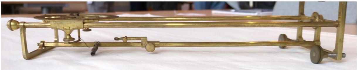
Fig. 4: Hair hygrometer, left side, in lying position (which is not the intended one for using the instrument). Source: Deutsches Museum (inventory number 128). Photograph taken by the author.
