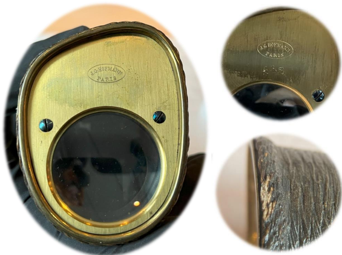
Fig. 4 Close-ups of three different details of the objective plate. Clockwise: the brass plate with the screws and the inscription “J.G. HOFMANN PARIS”, the stain on the plate with the digits “6 3 9” clumsily engraved, and the scratches on the edge of the woven cover. Source: Deutsches Museum Munich, © Photographs by Luisa Lovisetti.
