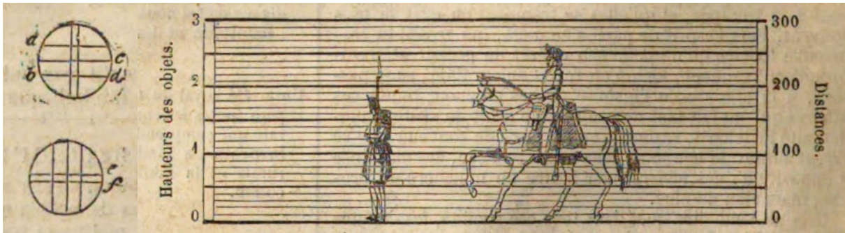
Fig. 10 The two possible wire reticules (the second is simply the first one rotated by 90 degrees) and the comparison scale for measuring distance. (Anonymous 1850: 288)
