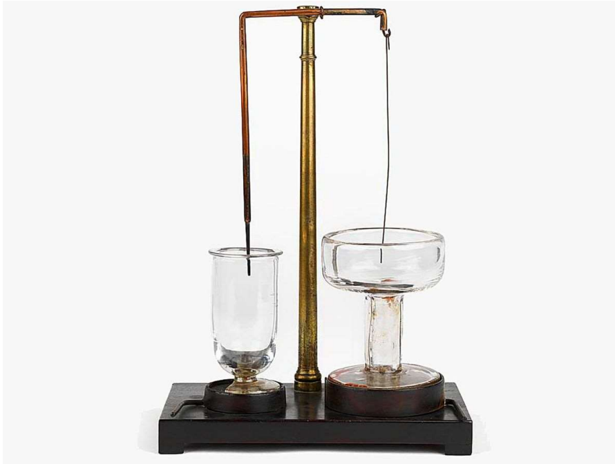
Fig. 6 Faraday's original rotation apparatus. Source: Royal Institute.
