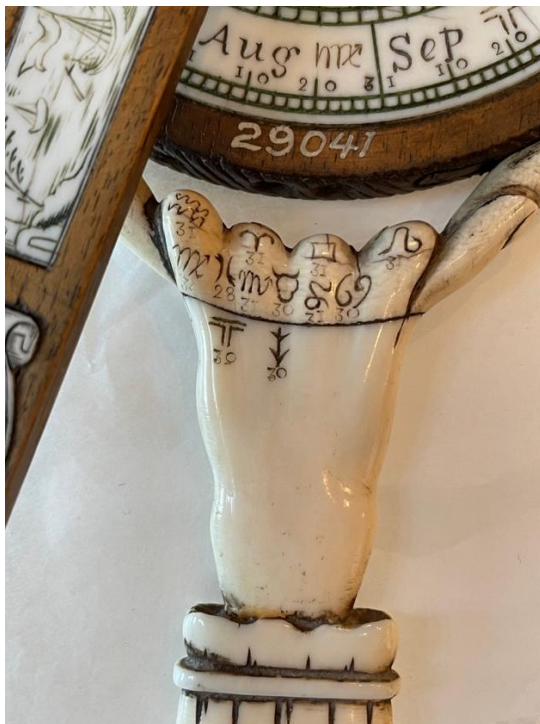
Fig. 21 Close up of the hand attached to the bottom disk of the nocturnal. Source: Deutsches Museum, Munich. Photography by author.
