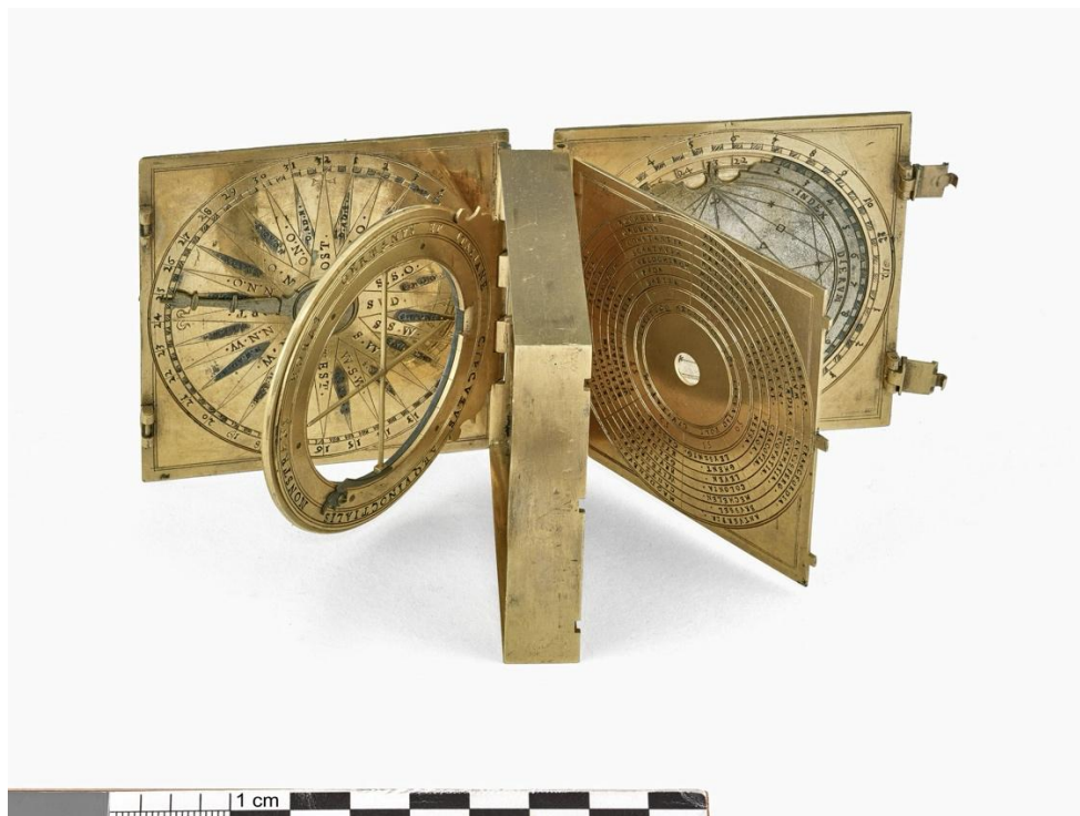
Fig. 7 Astronomical Compendium with equatorial sundial. Caspar II Buschmann, Augsburg, ca. 1560–1613. Source: Deutsches Museum, Munich, Inv.-Nr. 43553 © Konrad Rainer (CC BY-SA 4.0).
