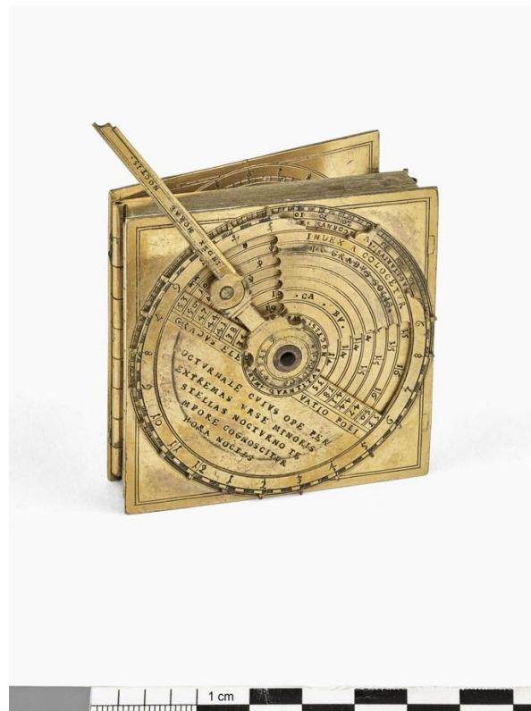
Fig. 8 Frontside of the compendium in Fig. 7, showing a nocturnal with its index arm protruding out. Source: Deutsches Museum, Munich. © Konrad Rainer (CC BY-SA 4.0).
