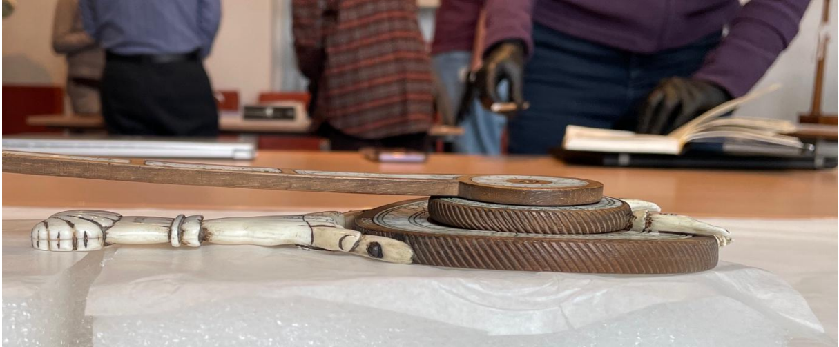
Fig. 10 Side view of the nocturnal, showing how the three discs are stacked on top of each other. Source: Deutsches Museum, Munich. Photograph by author.
