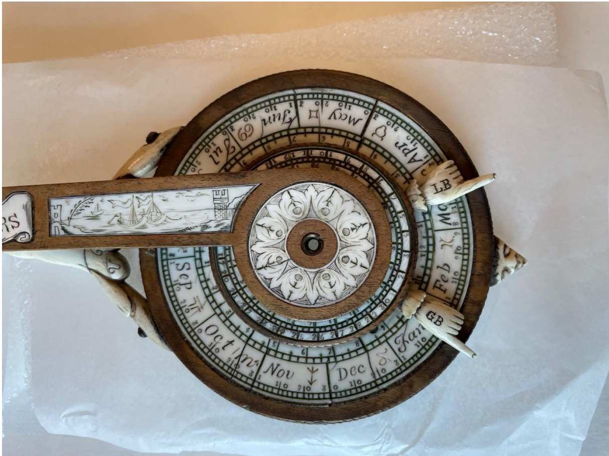
Fig. 12 Close up of the front of the nocturnal, displaying the three concentric disks. Source: Deutsches Museum, Munich. Photograph by author.
