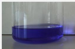
Abb. 3: Alizarin in NaOH
