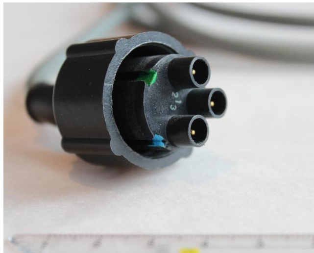
Fig. 3 Laser male plug with three connectors. Source: Deutsches Museum Munich © Miguel Teixeira.
