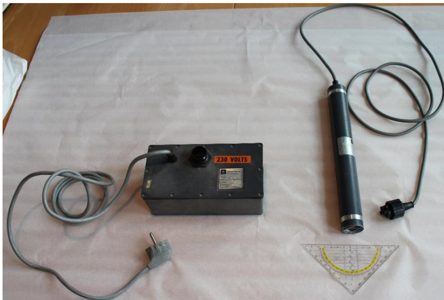
Fig. 2 He-Ne Laser and power supply/exciter. Source: Deutsches Museum Munich © Miguel Teixeira.
