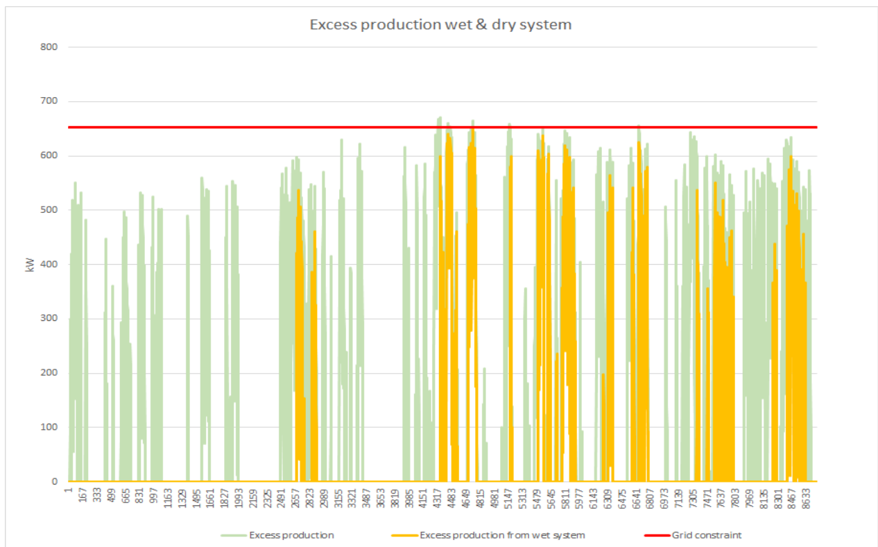
Figure I. 2. Excess generation into the local grid
