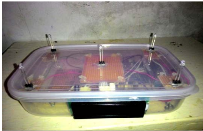
Figure 3. Solar radiation sensor from photodiodes
